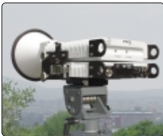
2GHz Transmitter Unit (TXU) with High Power Unit (HPU)
