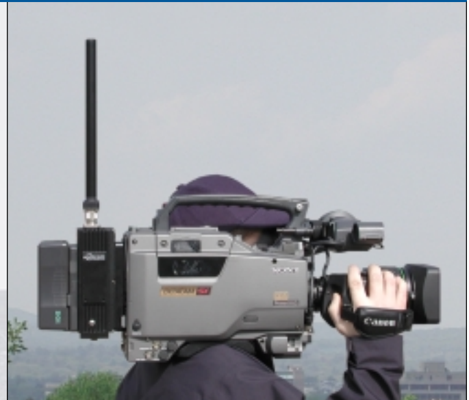
REPORTER Camera Mounted Transmitter using an integrated V-Mount design
