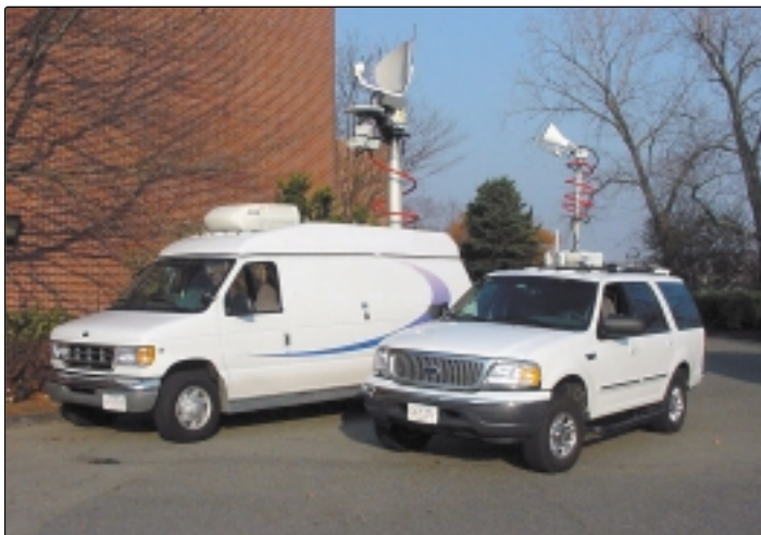
CodeRunner 2 in existing van installation (left). SUV Installation with Omni Directional and MegaHorn Antenna (right)
